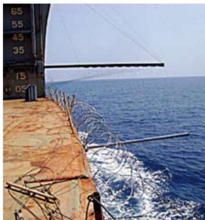
**WHILE some owners are using armed guards, other are installing sophisticated passive defence systems such as the P-Trap® (above) which creates a safety zone around the ship. The trap is a boom that is extended from the bow of a vessel on both sides. P-Trap® lines are installed on the boom which float just below the surface of the water and disable pirates' engines by trapping the propellers. The line will then break and pirate vessels will be left floating and inoperable.**
